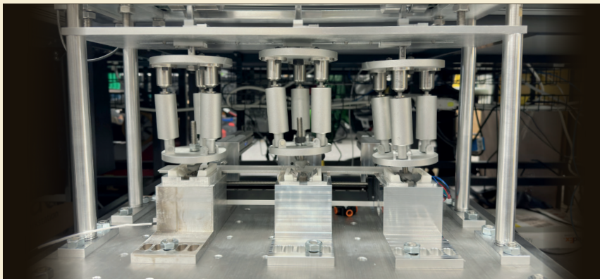
The TriChewer, a mechanical chewing model.
